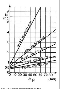
Fig. 7a Power consumption of the RUVAC WS/WSU
