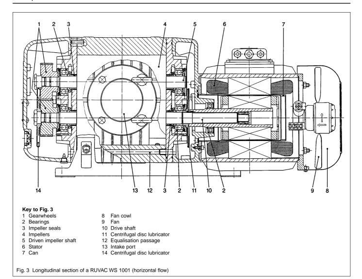
RUVAC pumps from the WS/WSU range have been specifically designed for operation in the rough and fine vacuum ranges. They are thus either used in connection with backing pumps or in closed gas cycles. The pump's power consumption depends not only on the pumping chamber volume and the rotational speed of the pump, but also on the pressure differential between the discharge and intake flanges (see Fig. 7).
