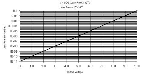
Figure 3-10 Leak Detector Logarithmic Output Voltage
