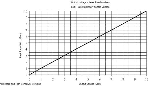
Figure 3-9 Leak Detector Linear Output Voltage
