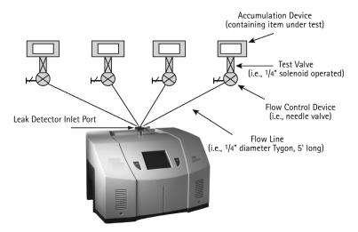
Figure B-7 Accumulation: Inside Out
