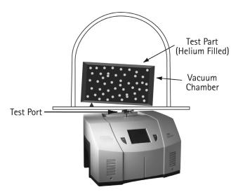
Figure B-5 Measuring Leaks: Inside Out
