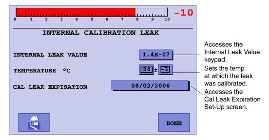
Figure 3-17 Internal Calibrated Leak
