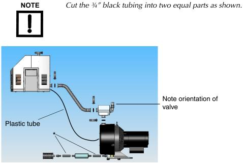
Figure 1-11 Bench Mount Leak Detector with External TS620 Dry Scroll Pump, Model VS BD30+
