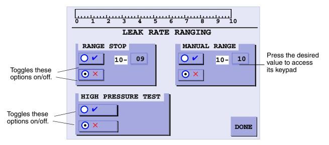
Figure 2-12 Leak Rate Ranging
