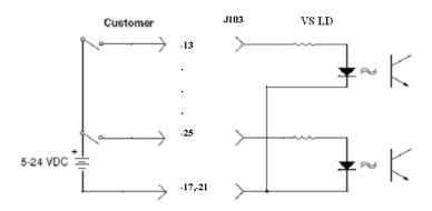
Figure A-3 Optically Isolated Input Circuit Sketch
