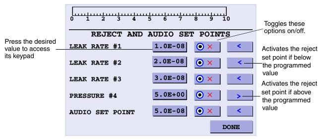
Figure 2-10 Reject and Audio Setpoints
