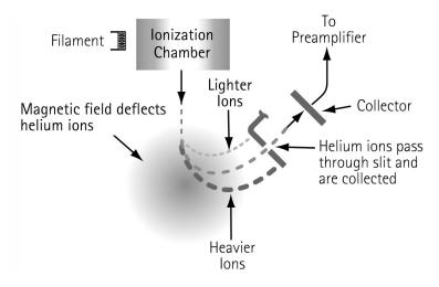
Figure B-1 Magnetic Separation Principle
