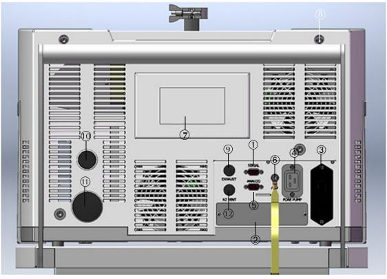
Figure 1-15 VS Series Rear Panel
