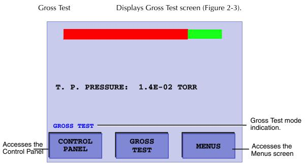
Figure 2-3 Gross Test Screen
