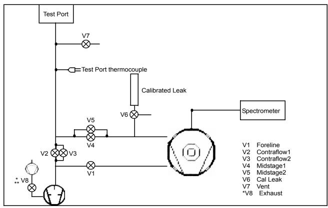
Figure 3-7 Leak Detector Vacuum System Diagram
