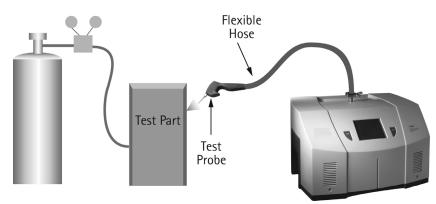
Figure B-6 Locating Leaks: Inside Out
