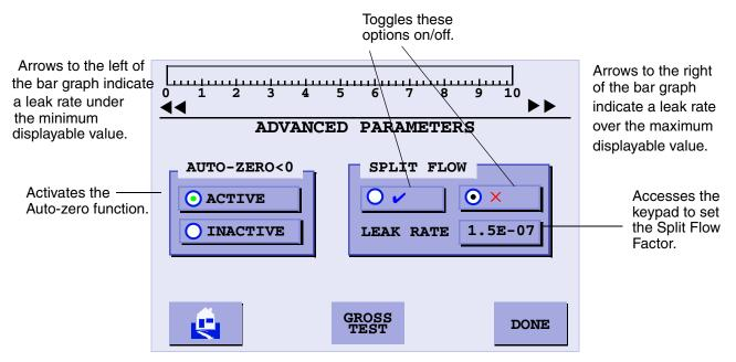
Figure 3-3 Advanced Parameters
