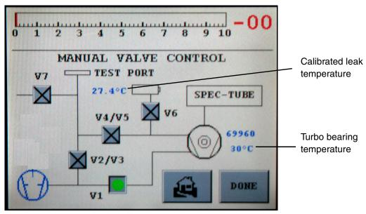
Figure 3-5 Manual Valve Control
