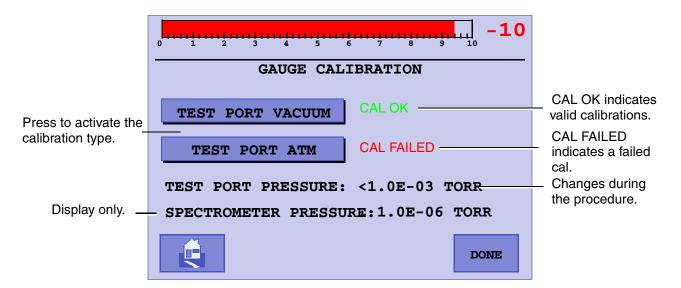
Figure 3-13 Gauge Calibration
