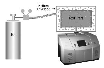
Figure B-4 Measuring Leaks: Outside In
