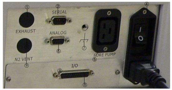
Figure 1-17 Rear Panel (with Discrete I/O PCB)
