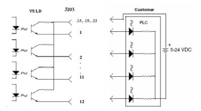
Figure A-2 Optically Isolated Output Circuit Sketch
