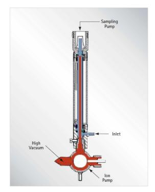
Figure B-2 Selective Ion Pump Detector
