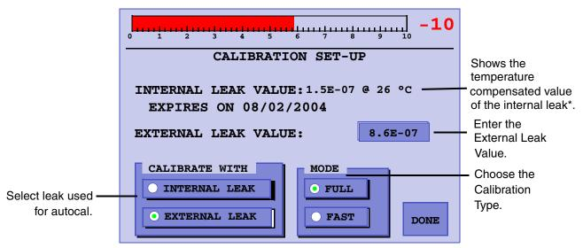
Figure 2-8 Calibration Set-Up
