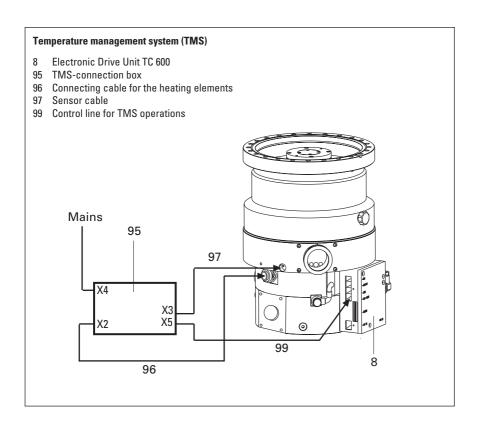
For connection and operation of the temperature management system (TMS) please refer to operating instructions for the TMS, PT 0099 BN.
