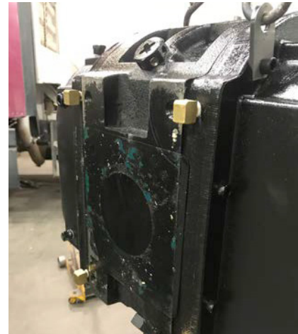
Figure 4-4 – Alternate plug configuration: Horizontal mount with street elbows
