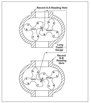
Figure 6-4 – Checking Rotor Interlobe Clearance
