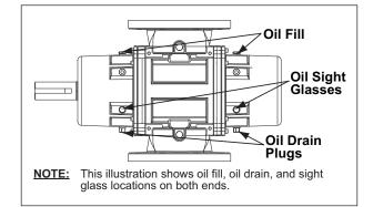
Figure 3-5 – Locations of Oil Fill, Oil Drain Plug, and Oil Sight Glass
