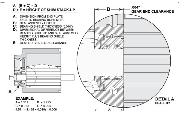
Figure 6-5 – Bearing Bore Stack-Up and Seal Measurement
