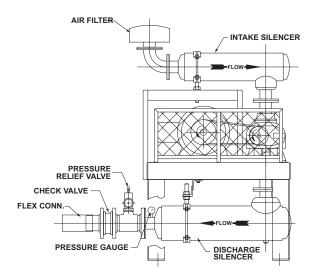
Figure 5-1 – Typical Blower Installation
