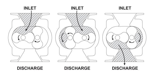
Figure 4-1 – General Operation Principle
