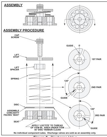
Figure 6. Discharge Valve
