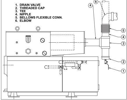
Figure 4. Flex Connector Configuration
