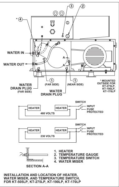
Figure 5. Water Miser and Heater Installation
