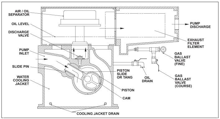
Figure 1. Cross Section of Pump
