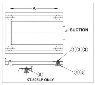
Figure 2. Vibramount Positioning
