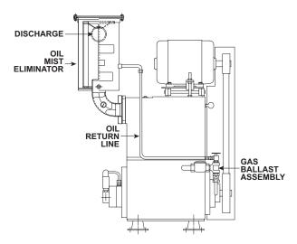
Figure 5-2 - Oil Return to the Gas Ballast Valve
