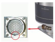
2 - Then identify the main index on the cable connector.
