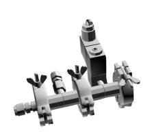
This valve will slow down the pump in complete safety. With this option, the braking time from nominal speed to 0 rpm is t < 15 mn. Without this accessory, the braking time is about 30 mn. (See **B** 40 for valve installation).
