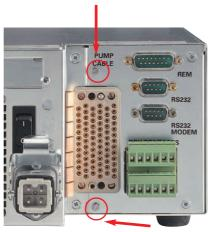
If you fail to remove the 2 screws, you will not be able to insert the connector, fully: that may cause electrical damage to the controller.
