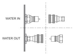
Fig. 6: Water circuit connection
