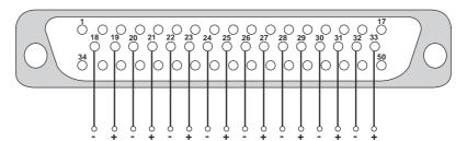
Fig. 13: J1 connector: control with DC voltage
