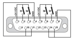
Fig. 17: J4 connector: digital input wiring
