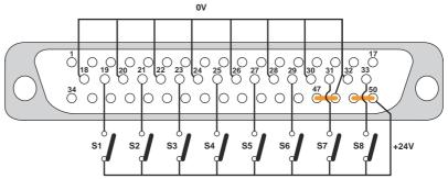
Fig. 14: J1 connector: control with dry contacts
