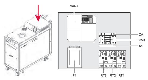
Fig. 29: Location of electrical components: pump with one frequency converter VAR1 Frequency converter Current sensor Α1 F1 Power filter RT1 FB circuit breaker CA Auxiliary contact RT2 Roots circuit breaker KM1 RT3 FB command Heating circuit breaker (option)
