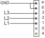
Fig. 8: Main supply connection
