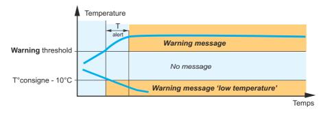
The heating system is equipped with a thermal safety which cause a fault in case of overload. A warning appears. A delay can be set for a pre-alarm: [SETTING] [TEMPERATURE] [HEATER ALARMS] [DEFAULTS] [PRE-ALARM] [ENABLED] [DELAY].
