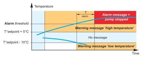
This monitoring is possible once at least the setpoint temperature is reached. Otherwise the valve remains closed and the temperature faults are not managed.
