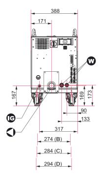
Fig. 23: A 124H, A 204H, A 204X - Dimensions (mm)
