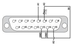
Fig. 16: J3 connector: analog output wiring
