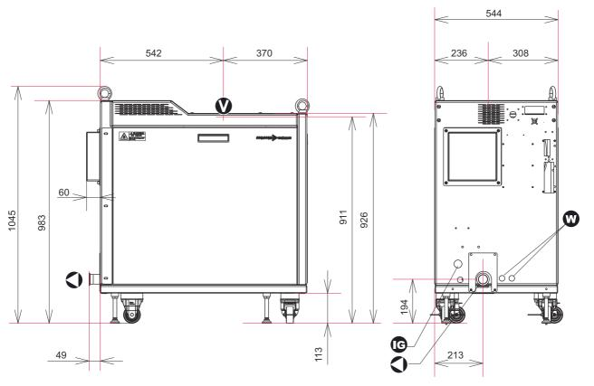
Fig. 26: A 2404H, A 2404X - Dimensions (mm)
