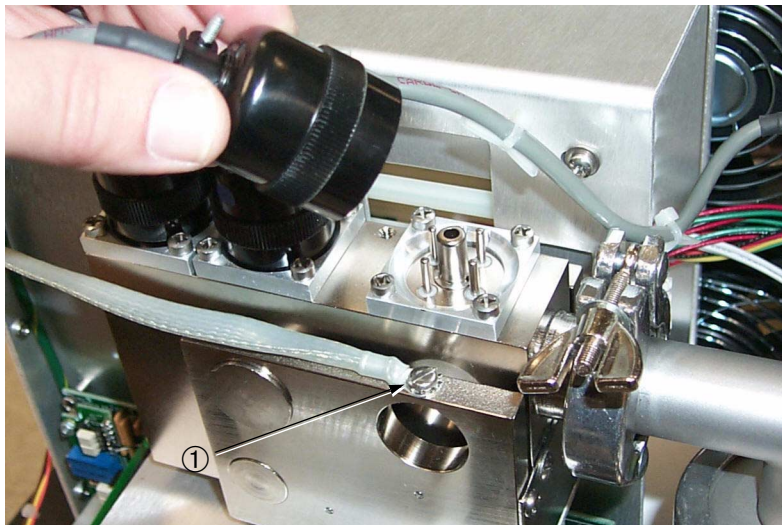
Figure 4-3 Removing the Connectors
