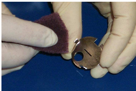
Figure 4-20 Discolored Ground Slit Plate
