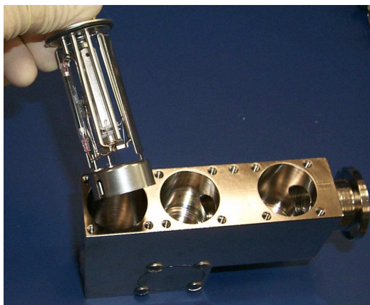
Figure 4-16 Removing the Preampifier
