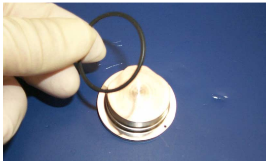
Figure 4-18 Removing the O-ring from Magnetic Pole Piece
