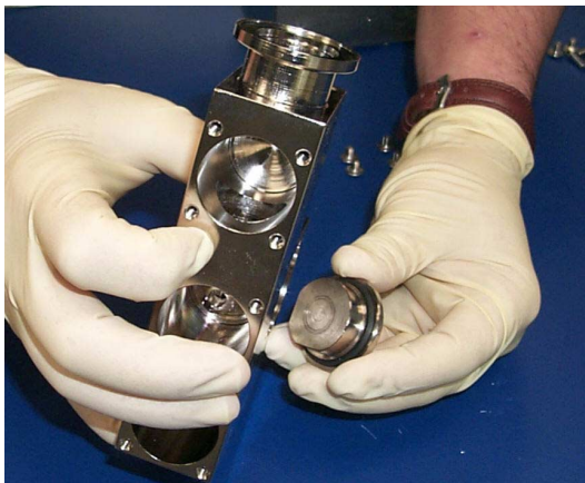
Figure 4-19 Removing the Second Magnetic Pole Piece
