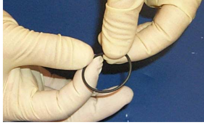
Figure 4-23 Inspecting the O-ring
