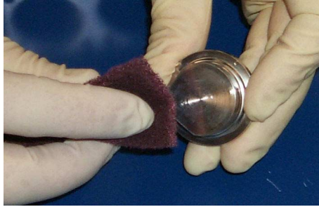
Figure 4-21 Discolored Ground Magnet Pole Piece
